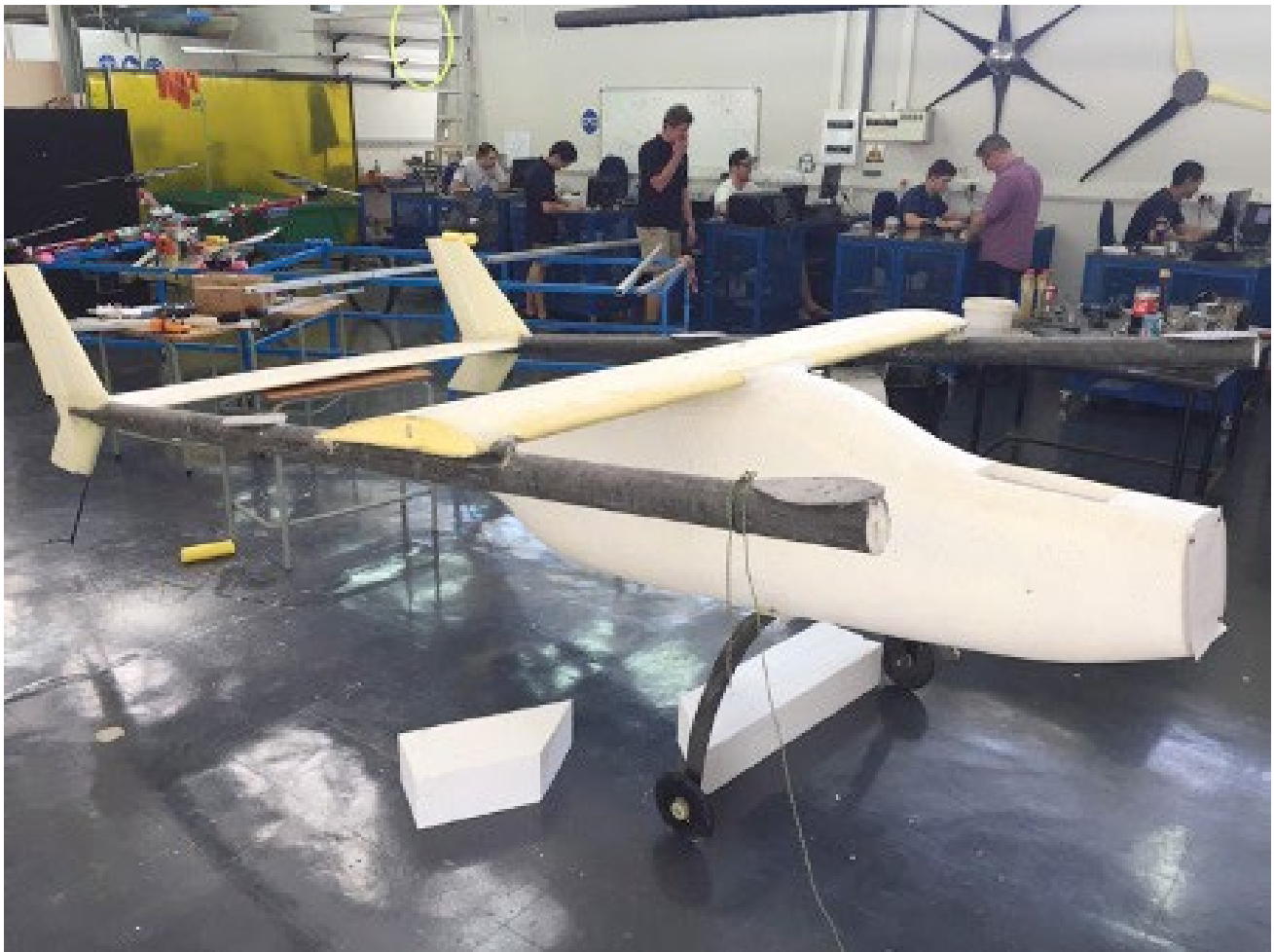
Nelson Mandela University prototype under construction (7,5m wingspan)
