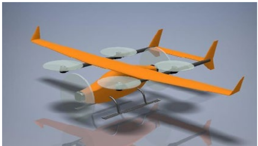
Forward flight mode – central motors provide forward thrust. Outer motors switched off and locked.
